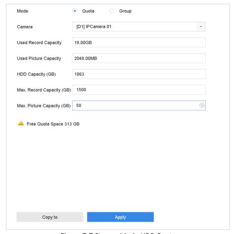
Figure 7-7 Storage Mode-HDD Quota
