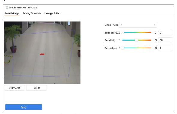
Figure 13-5 Intrusion Detection
