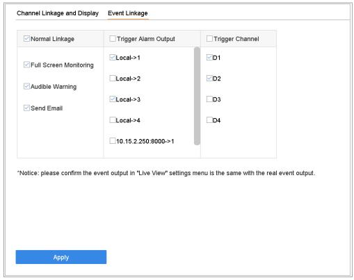
Figure 12-8 Set Trigger Cameras of POS
