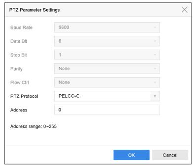
Figure 6-2 PTZ Parameters Settings
